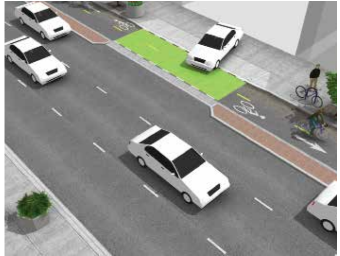
Two Way Cycle Track (Protected bike lane) - design credit: NACTO
