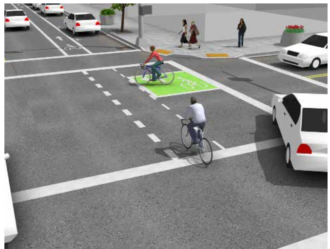
Two Stage Turning Movements - design credit: NACTO
