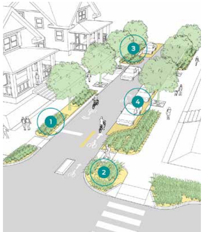
After - Residential street with stormwater plantings. 1. planting strip. 2. bike boulevard; curb extensions. 3. Mid-block extension. 4. Permeable pavement blocks. www.nacto.org
