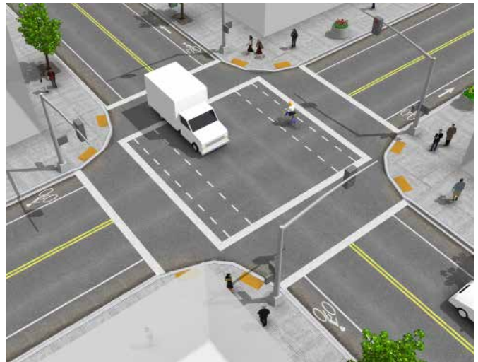
Bike Lane Intersection Markings - design credit: NACTO
