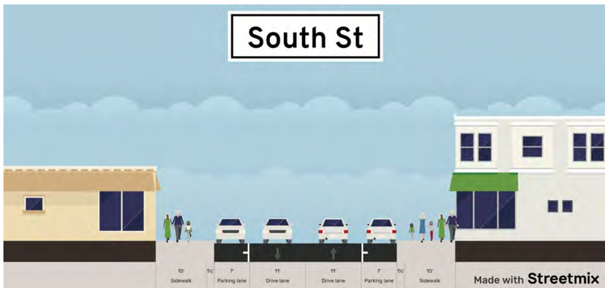
Figure 6-2: Proposed Cross Section for South Street from Westnedge Avenue to Portage Street
