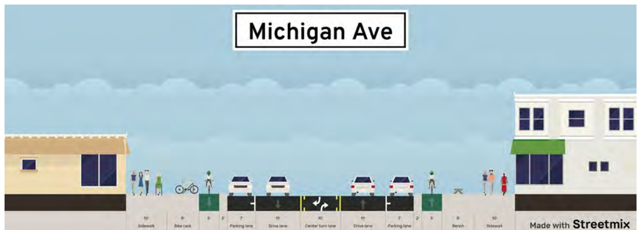
Figure 2-4: Proposed Cross Section for Michigan Avenue with Bike Lanes at the Sidewalk Level
