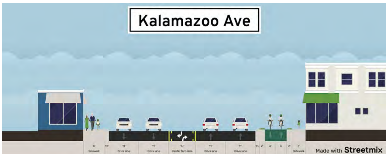
Figure 3-3: Proposed Cross Section of Alternative #1 for Kalamazoo Ave
