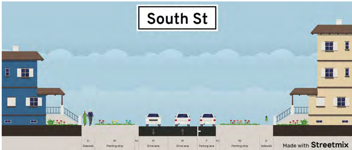
Figure 6-3: Proposed Cross Section for South Street from Michigan Avenue to Westnedge Avenue
