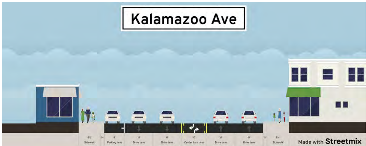
Figure 3-5: Proposed Cross Section of Alternative #3 for Kalamazoo Ave
