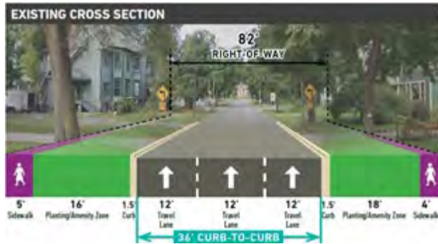
Figure 8-2: Existing Cross Section of Douglas Avenue
